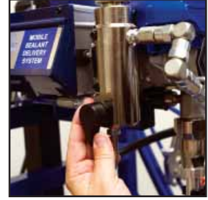
Turn prime valve down slowly to direct product through prime tube.
