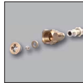
Remove flat washer, ball bearing and clover leaf bearing from lower pump housing and clean each part. Reassemble.
