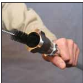
Clean siphon tube with brush and reassemble.
