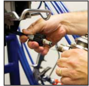
Remove the pressure hose from the lower pump assembly.
