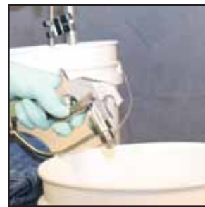
Spray until water runs clear from pump and hose by triggering gun into empty pail.
