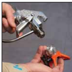
Remove tip guard assembly.
