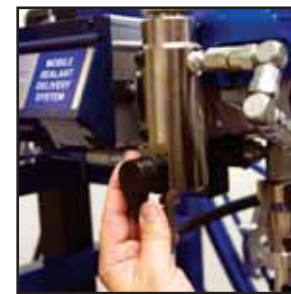
Turn prime valve down and allow flushing fluid to circulate for 15 to 30 seconds to clean drain tube.
