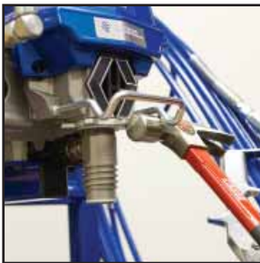
Loosen threaded nut on pump housing.
