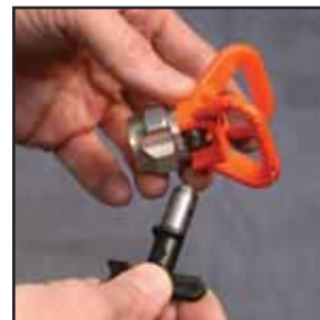
Remove reversible spray tip and bushing to clean with water.
