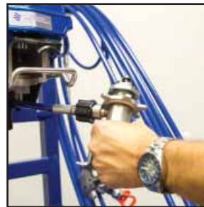
Remove the lower pump assembly.
