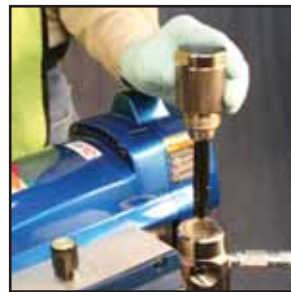
Remove cap from fluid outlet housing.
