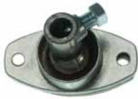
An economical zinc alloy die cast fitting, which firmly clamps the control rod from a splitter damper bracket as it extends through the duct. Comes completely assembled with set screw, neoprene back-up gasket and nylon cup washer which holds the ball firmly against the duct, preventing rattles.
